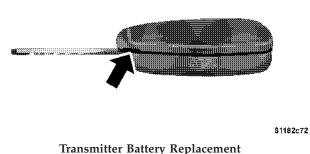
The recommended replacement battery is a 3V lithium 2016 cell. This transmitter requires two batteries.
